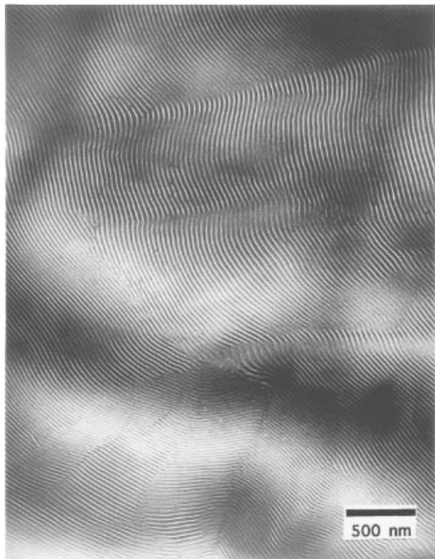
Figure 7. TEM micrograph of the lamellar morphology produced by the H material.
