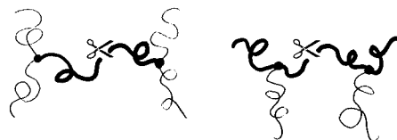
Figure 8. Formal division of the \pi and H molecular architectures into component simple graft block copolymers for the purpose of mapping the morphological behavior onto the simple graft morphology diagram.
